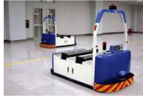
(b) Mobile feeding robot for feeding of a static container system.
