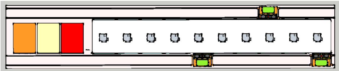
Figure 3.3: Schematic of a cell-based insect production facility where the cells are handled by robots (shown in green) from both the back and the front. Courtesy of Inagro, Sirris and Vives (Schillewaert et al., 2016).
