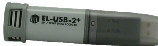
Figure 3-19: RH and temperature data logger of type EL-USB-2+
