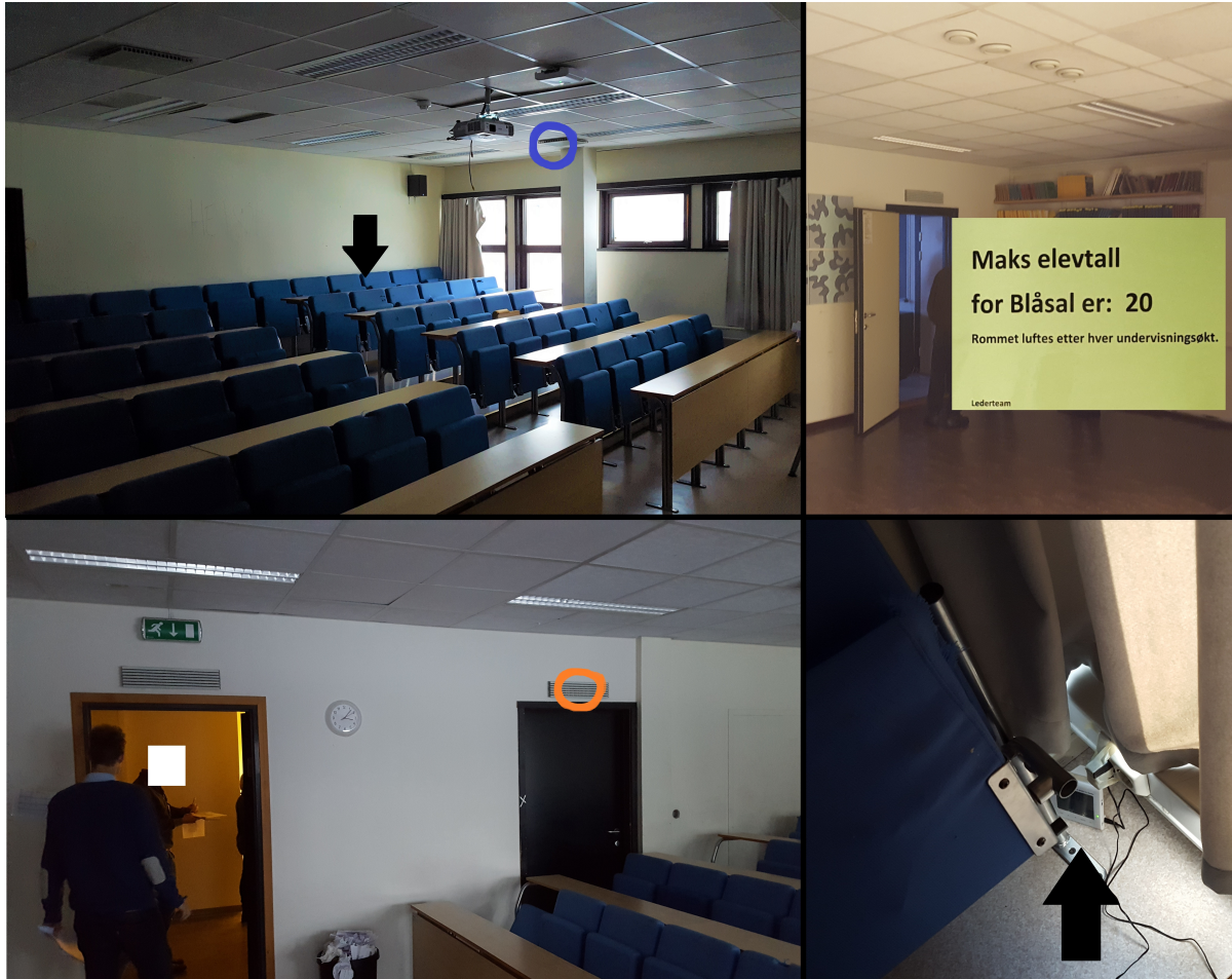
Figure 12: Pictures from the Room Blåsal. The top right picture is taken from outside the room towards the entrance door. The green screen was the poster pinned on the door. The blue circles shows the location of the supply air iButton and the orange circle show the extract air iButton. The black arrows show the placement of the ELMA monitor at the start and end of the field study.
