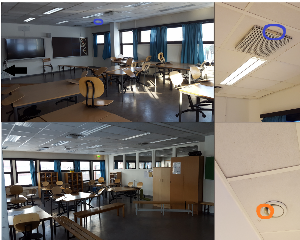
Figure 13: Four pictures from Room 321A at Stabbursmoen. The fresh air iButton is marked with a blue circle and the extract air iButton by an orange circle. The black arrow point to the placement of the ELMA monitor.
