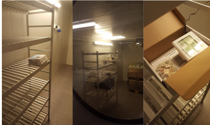
Figure 2: The leftmost picture shows the setup during the first session in the coldroom. The rightmost picture shows the cardboard seen in the leftmost picture. In the middle picture the setup for the second test session in the coldroom is shown. The large device seen is the Pegasor monitor.
