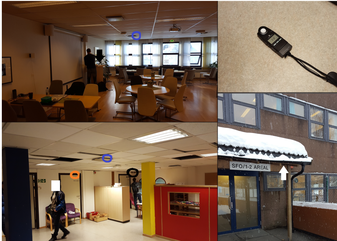
Figure 14: Four pictures from Stabbursmoen. The top left is from the Teacher's lounge, the black arrow shows the location of the ELMA monitor, beneath that is a picture from the SFO-room. The supply air iButtons are marked by the blue circles. The extract air iButton is marked by an orange circle. The top right show a light measurement done from the SFO room. The Bottom right picture shows where the iButton located outside was mounted, indicated by a white arrow.
