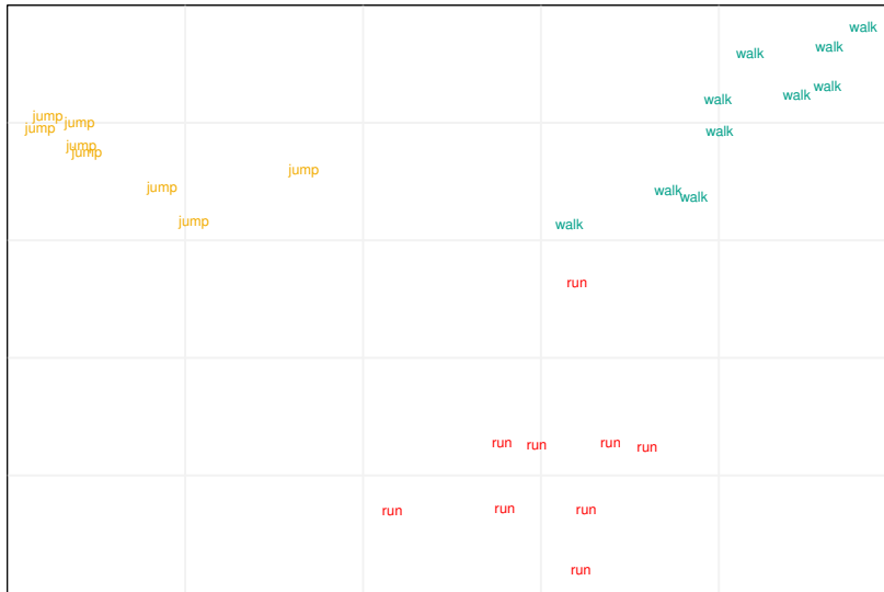
Fig. 9.7. Multi dimensional scaling plots of similarity matrix based on similarity measure \text{sim}^3 . In this plot we have taken animation with descriptions "run/jog", "forward jump" and "walk" from the CMU Motion Capture Database [13].
