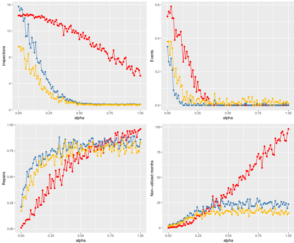
Figure 5.8: We run the adaptive method for \alpha \in [0, 0.01, 0.02, \dots, 1] to see how different \alpha values affect the outcome of inspection simulations with the three different strategies: non-adaptive (red), adaptive (blue) and VOI (yellow). For every \alpha we run 100 simulations with batch size 1. Clockwise from top left corner: Number of inspections against \alpha , number of events against \alpha , number of non-utilized months against \alpha and number of repairs against \alpha .
