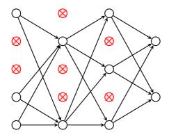
Figure 1.4: Visualization of dropout on three fully connected layers.
