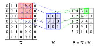
Figure 1.3: An illustration of a 2D convolution layer operating on a matrix input.
