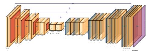
Figure 3.3: A 3D view of an UNet architecture. The numbers beneath each layer represents the number of filters in the convolution.
