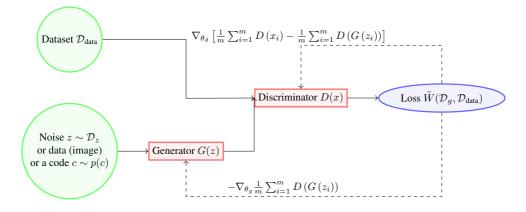
Figure 3.1: A basic setup for a Wasserstein GAN including the alternative gradients.
