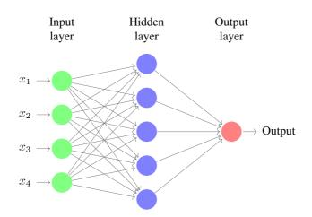
Figure 1.2: A visual representation of a one hidden layer fully connected neural network without bias vectors.
