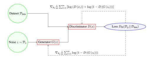
Figure 2.1: A basic setup for a generative adversarial model using the JS-loss.
