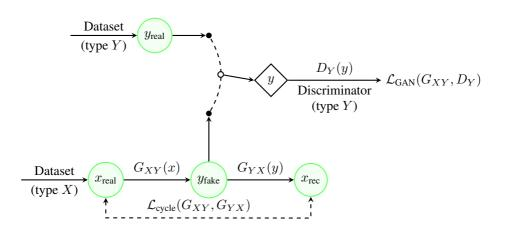
**Figure 3.4:** Visual representation of the  $X \to Y \to X$  cycle of the Cycle GAN. The  $Y \to X \to Y$  cycle is analogous to this just with X and Y flipped.
