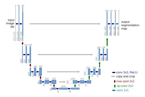
Figure 3.2: The UNet architecture from the original UNet paper on biomedical image segmentation.
