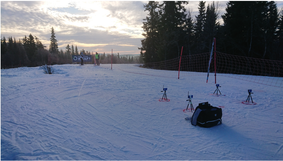
Figure 3.2: Photograph of the setup for estimating the friction coefficient. To the right are the four photo cells in one end of the setup, used to estimate the velocity in one end of the test track.
