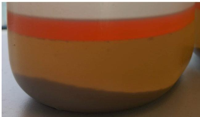
**Figure 3.2:** The received three fractions after hydrolysis was performed. From top to bottom: lipid fraction, aqueous fraction and sludge.
