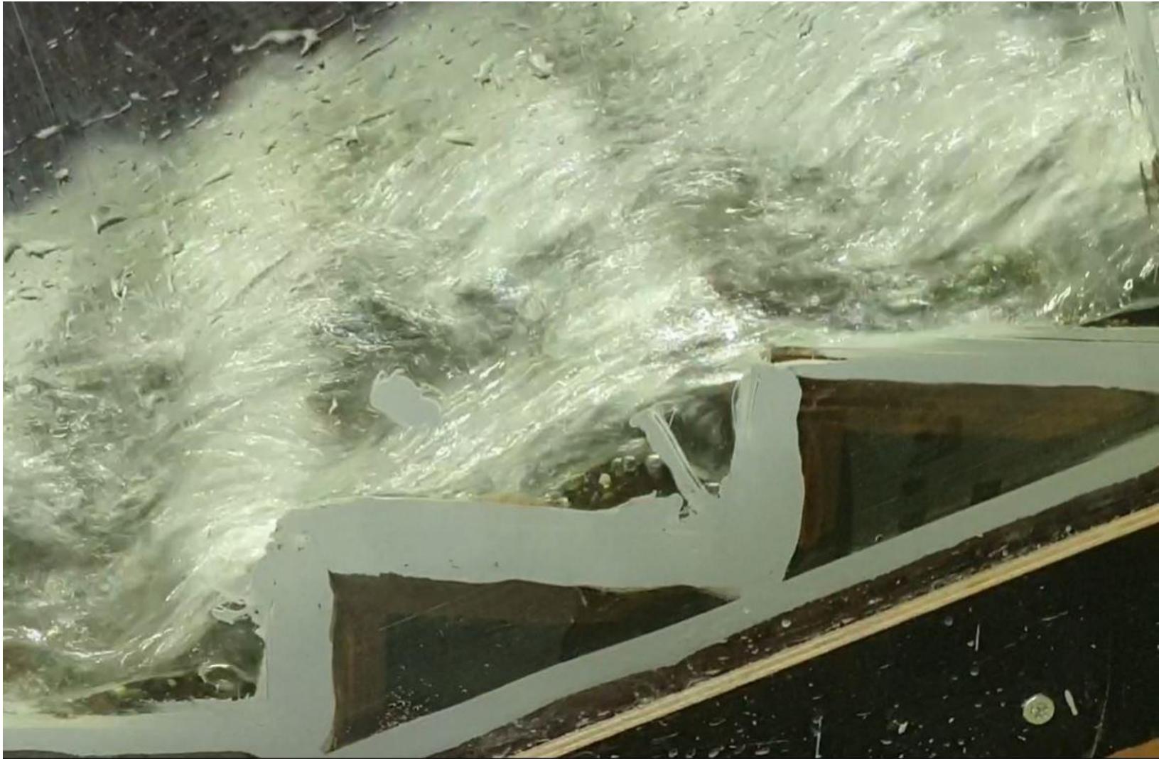
Figure 4: Low flow of 3.2l/s on step A. Partial jump taking place and air cavity beneath the falling nappe present
