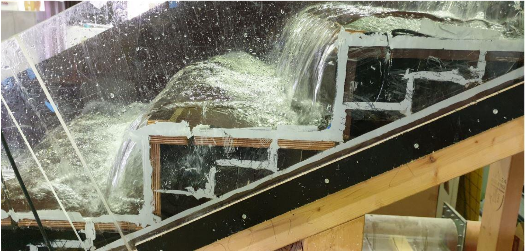
Figure 6: Fully developed hydraulic jump on step set C (Polled steps) at 3.2l/s
