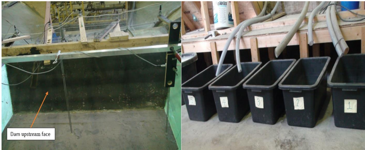
Figure 3-4 Photograph of the dam from the upstream side and the overtopping water collecting buckets
