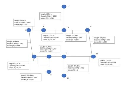
Figure 6.2: Grid properties for Loop structure
