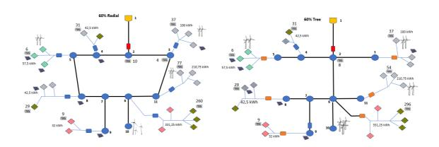
Figure 6.10: Battery placement and capacity 60 % RES both topology
