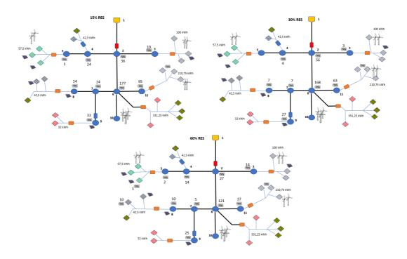
Figure 6.6: Battery placement and sizing 15,30 and 60 % RES Radial Tree grid
