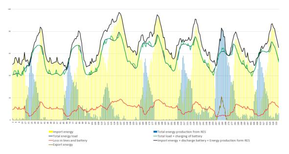
Figure 4.3: Energy behaviour from case 1
