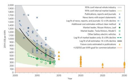
Figure 1.1: Projected costs for Li-ion batteries. Figure extracted from (Nykvist and Nilsson, 2015)
