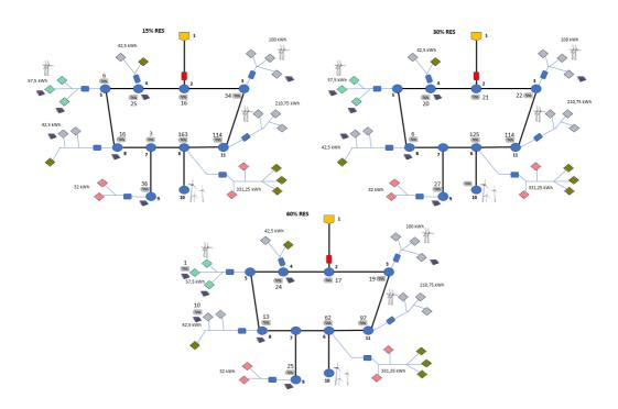
Figure 6.5: Battery placement and sizing 15,30 and 60 % RES in Loop grid
