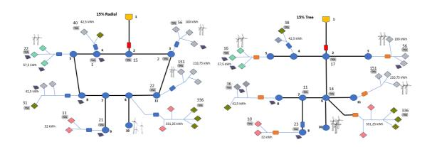
Figure 6.9: Battery placement and capacity 15 % RES both topology
