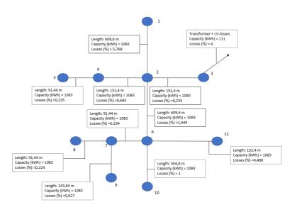
Figure 6.1: Grid properties for Radial Tree structure
