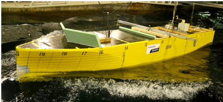
Figure 3-2 Model tested in the towing tank
