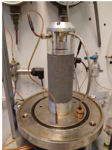
Figure 5.11: Preliminary bender element tests on the unconfined specimen
