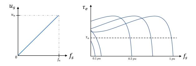
Figure 3.1: V/f curve without voltage boost
