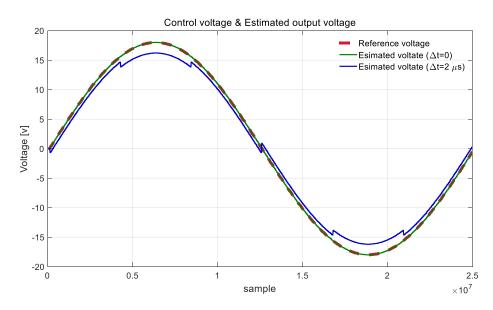
Figure 7.7: Simulation – Voltage estimation with and without blanking time
