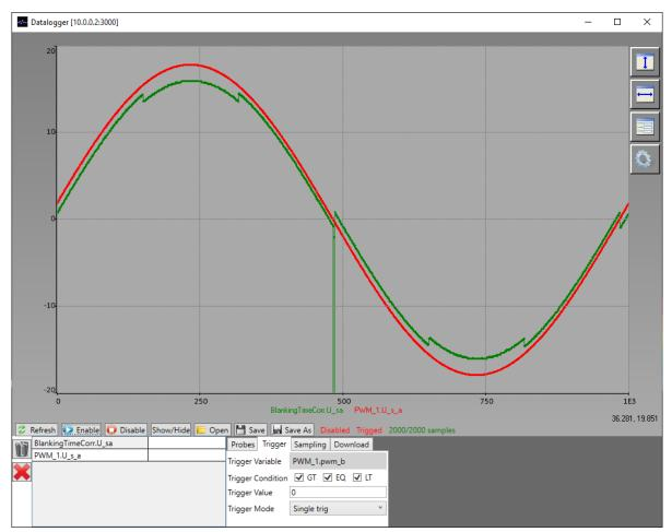
Figure 7.9: Control board – Voltage estimation with blanking time
