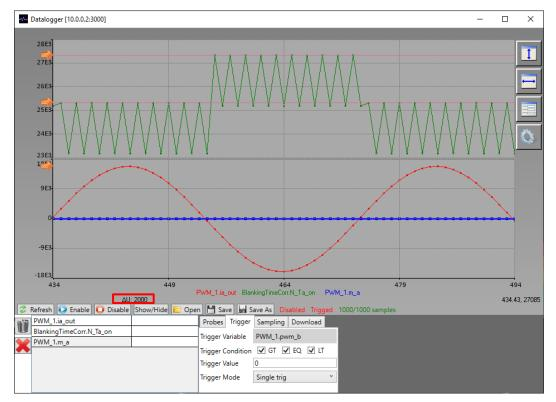
Figure 7.6 Control board - on-time count for DC-test with blanking time
