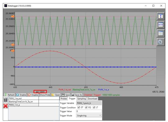
Figure 7.5: Control board - on-time count for DC-test without blanking time
