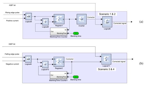
Figure 6.9: Blanking time correction of IGBT bit. (a) positive current. (b) negative current.
