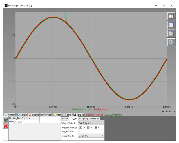
Figure 7.8: Control board – Voltage estimation without blanking time
