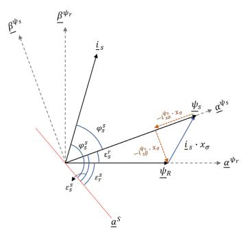
Figure 3.5: Vector diagram for used in voltage model
