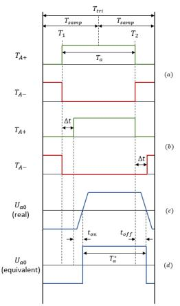
Figure 4.4: Switching patterns for a two level threephase inverter with current flowing to the load. (a) Ideal switching. (b) Switching this blanking time. (c) Actual phase to 0 voltage. (d) equivalent phase to 0 voltage
