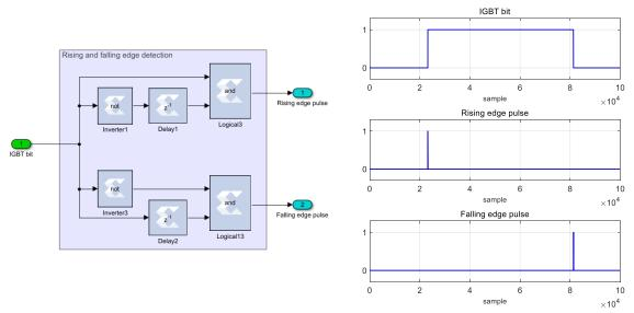
Figure 6.6: Rising and falling edge detector
