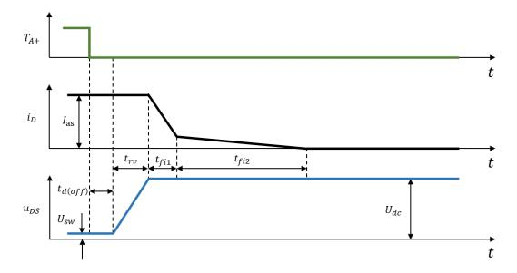
Figure 4.3: Turn-off voltage and current waveform
