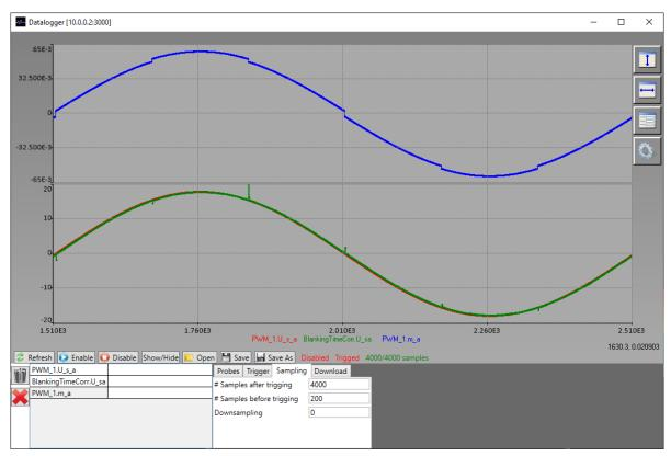
Figure 7.11: Control board – Voltage estimation with compensated control voltage
