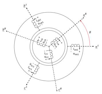
Figure 2.2: Schematic representation of the three-phase Induction Machine
