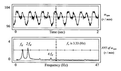
Figure 4.9: Mechanical speed and FFT analysis of mechanical speed with measurement errors [18].
