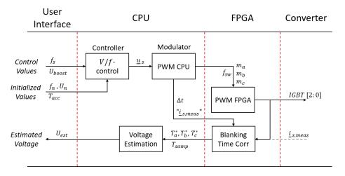
Figure 6.1: Objects and elements in the control software
