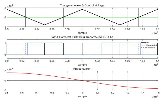
Figure 7.2: Illustration of Corrected and Uncorrected IGBT bit
