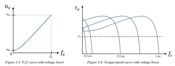
One method of avoiding the problem at lower speed operation and especially when the stator frequency is close to zero is to introduce a so-called voltage boost. The voltage boost compensates for the resistive voltage drop, ensuring a stator flux at 1 pu, thus making the machine able to produce the same torque throughout the nominal speed operation range. The voltage boost and the new torque/speed characteristic are presented in Figure 3.3 and Figure 3.4, respectively [16].
