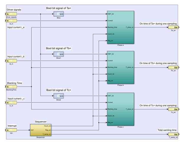
Figure 6.12: Complete block design of the blanking time corrector IP-core
