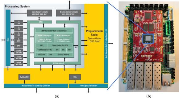
Figure 5.1: (a) schematic representation of the Zynq-processor [26]. (b) Photo of the control boards.
