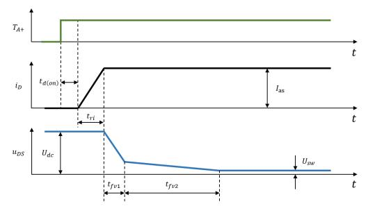
Figure 4.2: Turn-on voltage and current waveform
