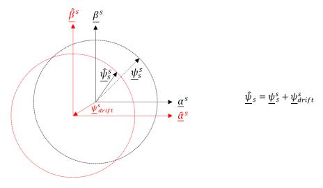
Figure 3.6: Drifting of stator flux
