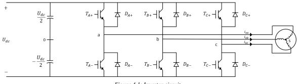
Figure 4.1: Inverter circuit
