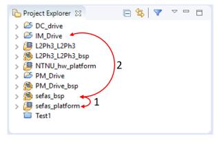
Figure 5.10: Link between hardware platform, BSP and project
