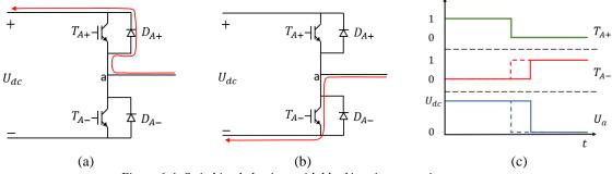
Figure 6.4: Switching behaviour with blanking time, negative current
