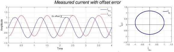
Figure 4.11: Offset error in current measurement
