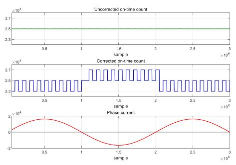
Figure 7.4: Simulation - on-time count for DC-test with and without blanking time
