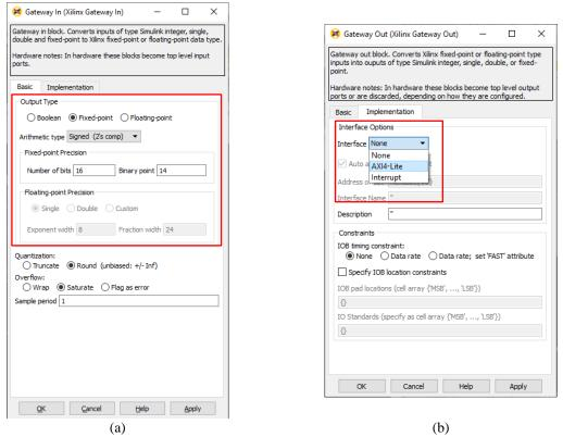
Figure 5.3: Block specification for Gateway ports
