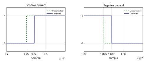
Figure 7.3: Close-up picture of turn-on and turn-off delay imposed by blanking time
