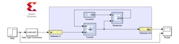
Figure 5.6: Simulation of counter
