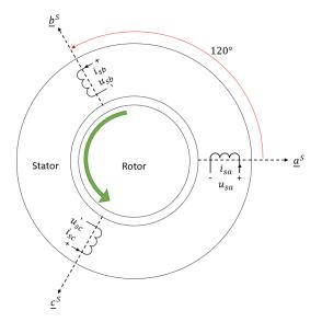
Figure 2.1: Principle drawing of the three-phase Induction Machine
