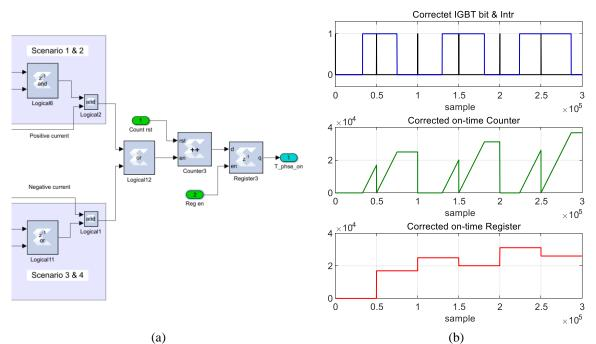
Figure 6.11: (a) counter and register logic. (b) corrected signal, on-time counter and on-time register
