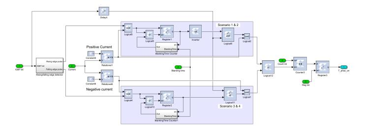
*Figure 6.5: Blanking time compensator*
