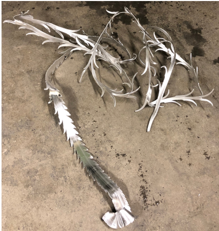
Figure 3.3: Full view of the torn profile.
