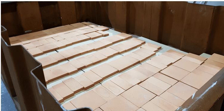
Figure 5.1: A photograph of one of the two anode containers which were used to pre-heat the carbon anodes. The anode container has been insulated in the bottom to reduce the heat loss to the ambient air outside the container. The bottom was insulated with a layer of heat resistant plates and then a layer of barrier bricks. During experiments, the space between the side walls and the anodes and butts as well as the top was insulated with Rockwool and insulating blankets.
