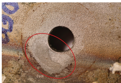
Figure 3.1: Corrosion attack under an artificial crevice former on the HAZ [90].
