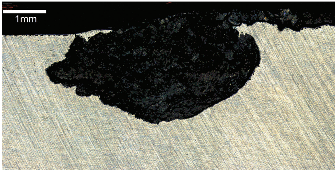
Figure 4.25: Cross-section of crevice corrosion attack on the TIG-welded, not pickled, coated Sample A which was polarized to +400 mV vs. Ag/AgCl, imaged by IFM.
