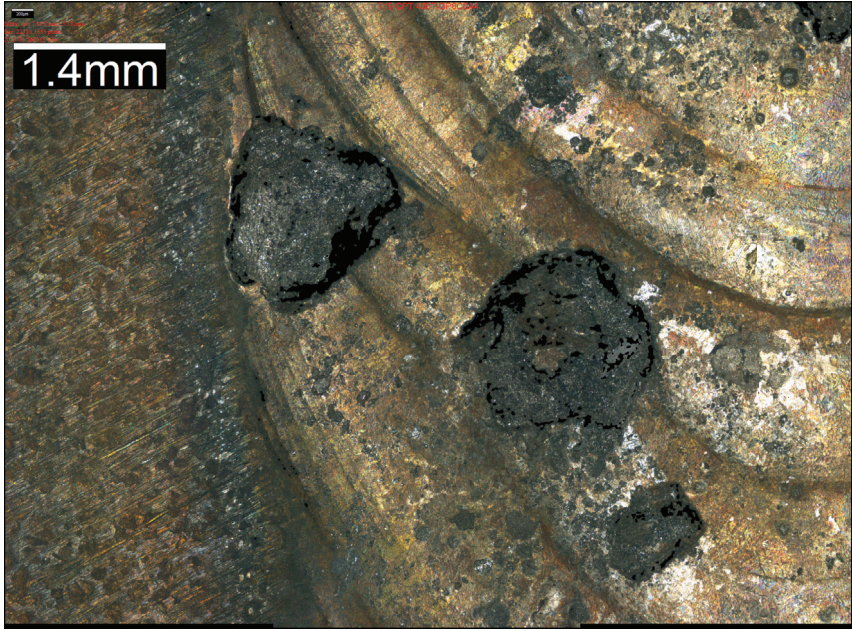
(a) IFM image showing corrosion attack.
