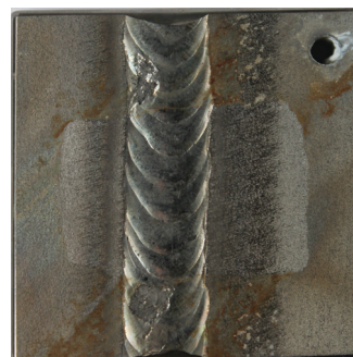
(b) Front side of coated sample.
