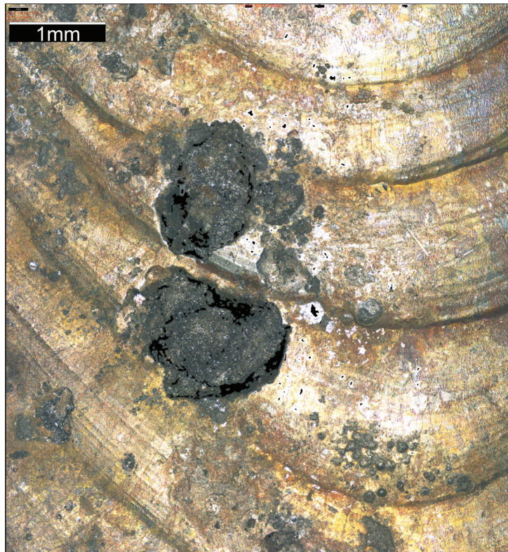
(a) IFM image showing corrosion attack.
