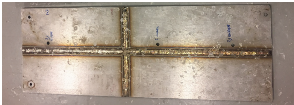
(b) Sample welded under high heat input without pickling.
