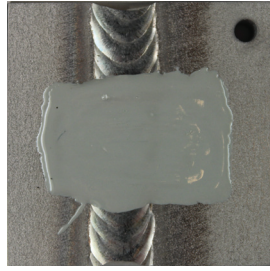
Figure 4.2: Coated TIG pickled sample.
