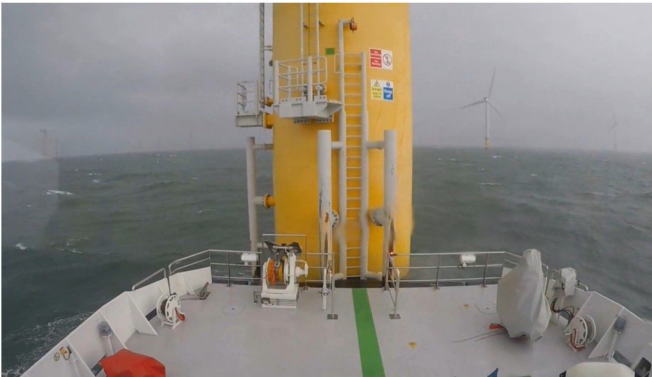
Figure 1.3: An Umoe Mandal vessel used for crew transport and boarding to an offshore wind turbine. Illustration by Umoe Mandal.
