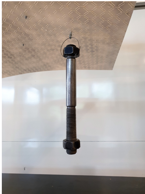
Figure 3.11: Load suspended from plate.
