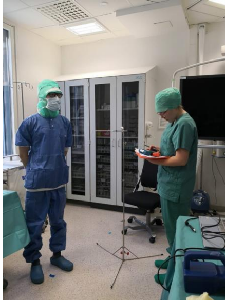
Figure 5 Air temperature and relative velocity measurements in OR
