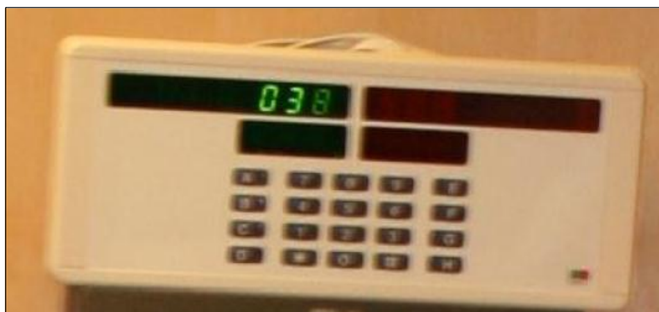
Figure A.3: Wall mounted display panel and the Imatis client (Sletten 2009).
