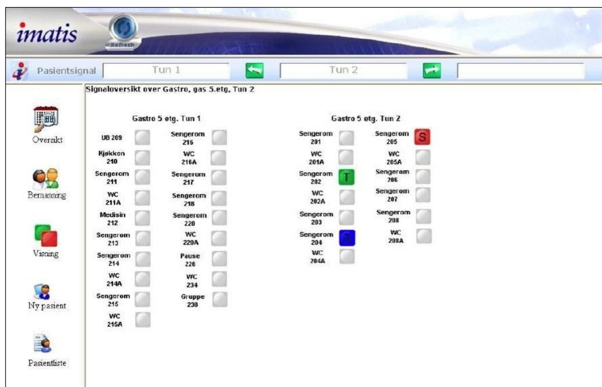
Figure 6.2: Imatis client GUI with a yet to be responded to assistance call on room #204 (slightly modified from Sletten 2009).
