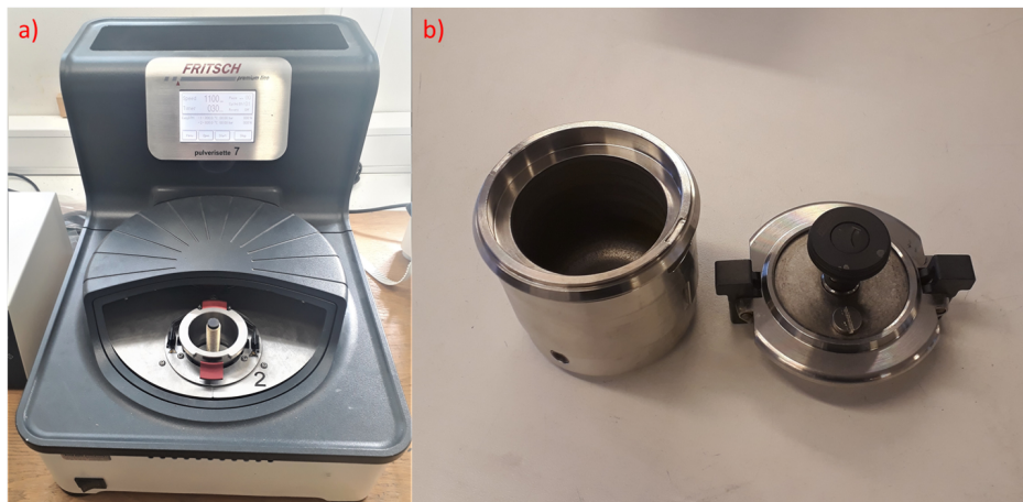
Figure 14: a) The Fritsch Pulverisette 7 Micro Mill used for ball milling. b) An example of the type of milling vial used during ball milling.
