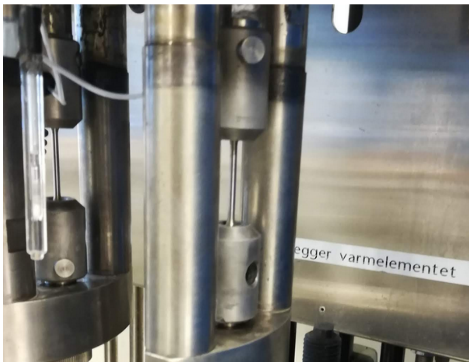
Figure 7: Slow Strain Rate samples of S235JR steel loaded into the Cormet prior to submersion in the MEA solution.
