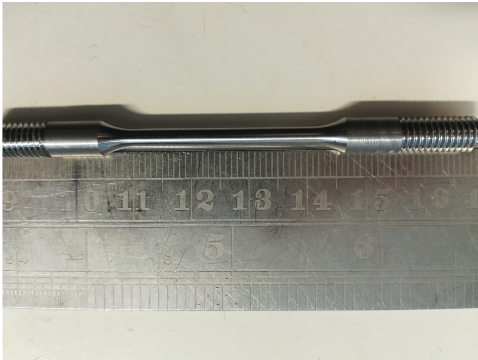
Figure 4: Stress test sample next to ruler.
