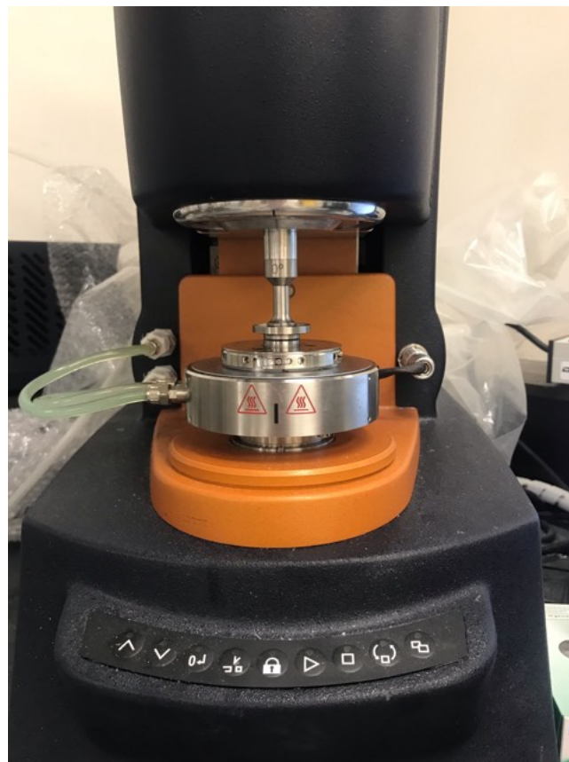
Figure 3.2: Discovery Hybrid Rheometer (DHR-3) with a 20 mm Peltier parallel plate geometry lowered to a 1000 \mu\text{m} gap thickness.
