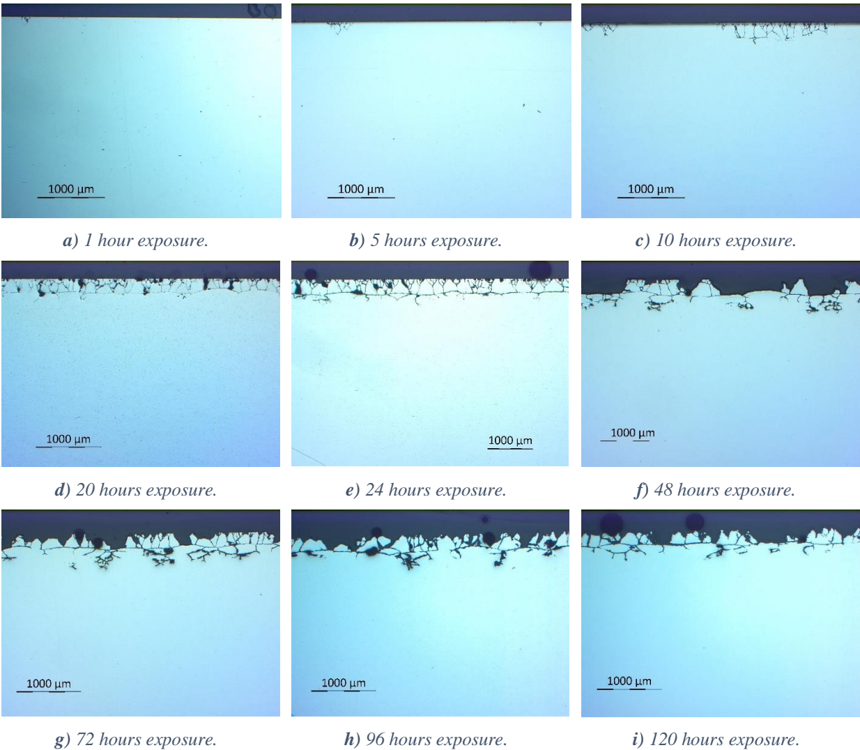
Figure 4.25 Corrosion of AA6005.40 T7 at varying exposure times. 25X magnification.
