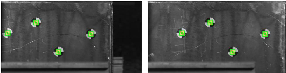
**Figure 2.5:** DIC of rigid body motion with subset tracking.
