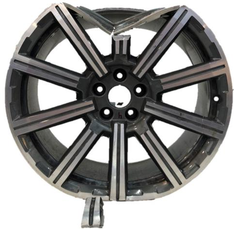
**Figure 6.45:** Images of all rims after testing. Impact from the bottom side of the images.
