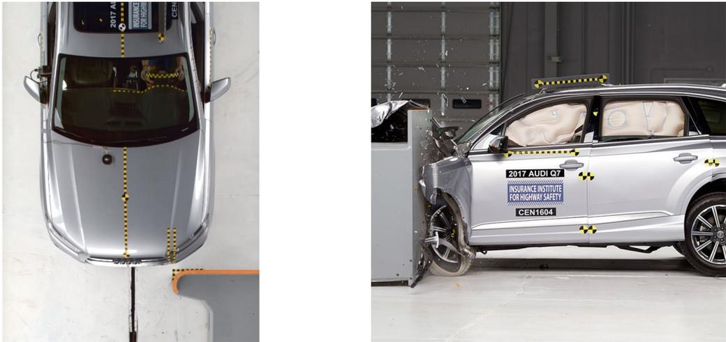
**Figure 1.1:** Small overlap crash test of the 2017 Audi Q7 [3].
