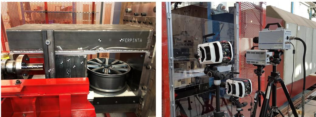
**Figure 6.13:** DIC overview and camera setup.
