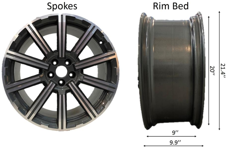
**Figure 3.1:** Front and side view of the Audi Rim.
