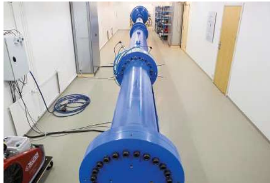
Figure 5.12: Picture of the shock tube, seen from the driver section. The picture is taken from [37].
