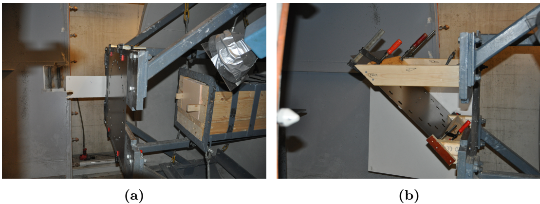
Figure 5.5: The two plate setups. (5.5a) Shows the orthogonal setup, and (5.5b) shows the setup which is tilted at an 45^\circ angle.
