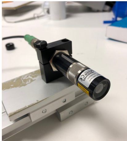
Figure 4.14.: Z-LASER Z185 line laser
