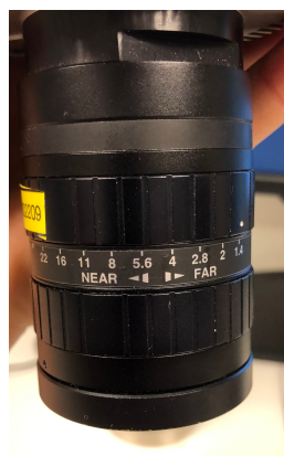
(b) Aperture increments on a FujiFilm CF16HA-1 lens
