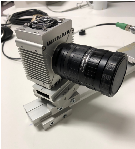
Figure 4.4.: AT C4-2040 CMOS sensor
