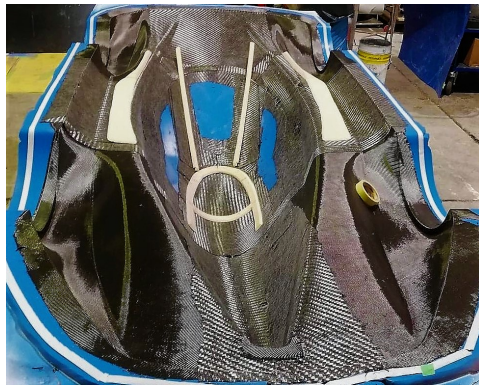
Figure 104: Core of upper body as it was manufactured
