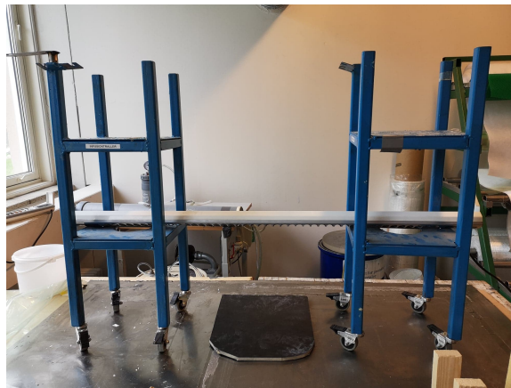
Figure 37: Epoxy curing at approximately 80 degrees Celsius
