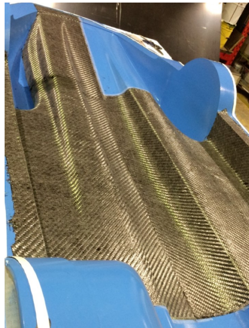
(b) Halfway through the first layer of the monocoque
