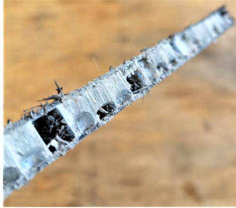
Figure 101: The cells of the honeycomb were saturated with epoxy, making the core heavier than PVC foam
