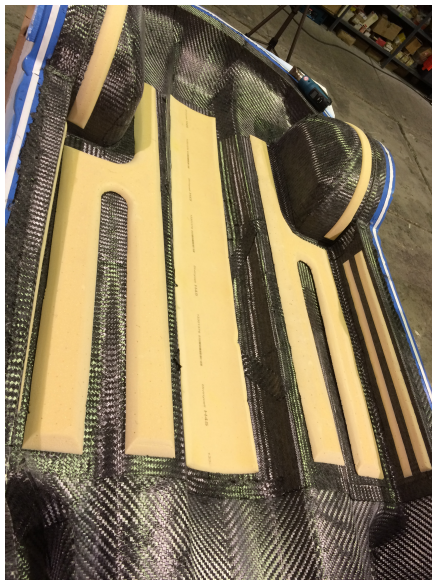
(a) The foam core on the lower body
