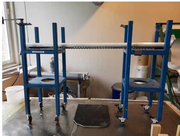
Figure 36: Epoxy curing at approximately 60 degrees Celsius
