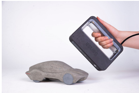
Figure 10: 3D-scanning of clay model
