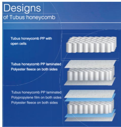
Figure 9: Three variants of Tubus honeycomb [28]
