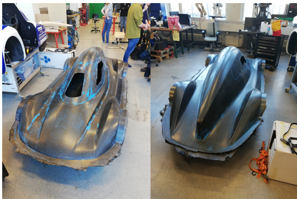
Figure 89: Top of the monocoque before post processing
