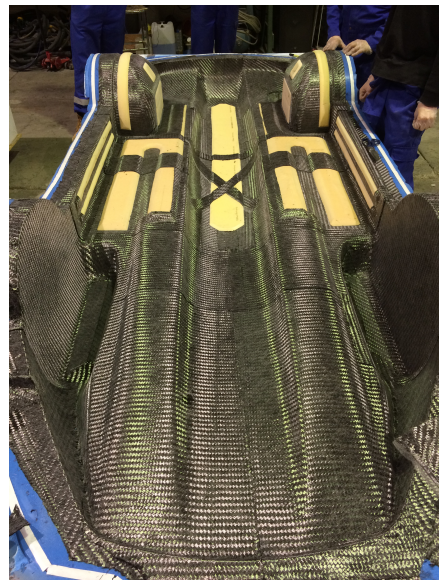
(b) First carbon fibre layer on top of the core
