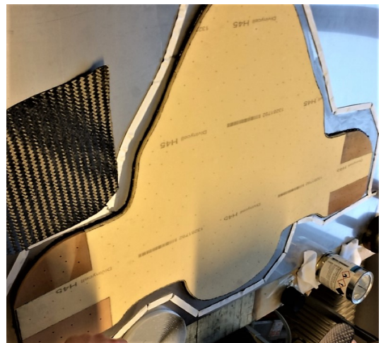
(b) Firewall. Notice the core in the corners is made denser to support the rear suspension
