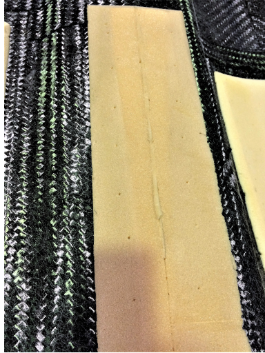
Figure 102: A wedge was placed in the middle of the core to bend it
