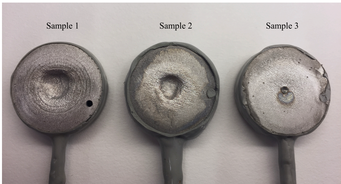
Fig. 5.38: The samples surfaces after the artificial pit experiment when the coating was removed.
