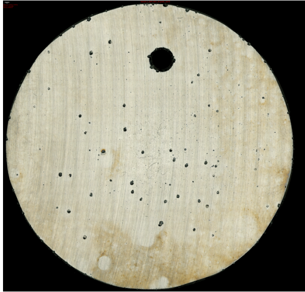
Fig. 5.6: The B-316L surface after anodic CPP in 5 wt% NaCl at 35 °C.
