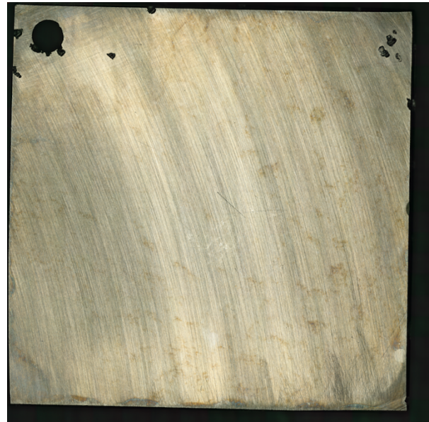
Fig. 5.8: The 316 Plus surface after anodic CPP in 5 wt% NaCl at 35 °C.
