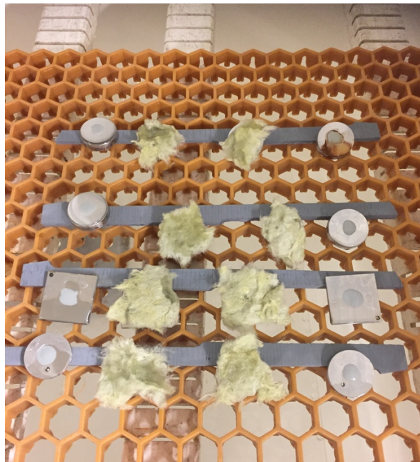
Fig. 4.8: The samples after 27 days in the salt spray chamber. Mineral wool was placed on selected samples and A-316L showed corrosion attack.
