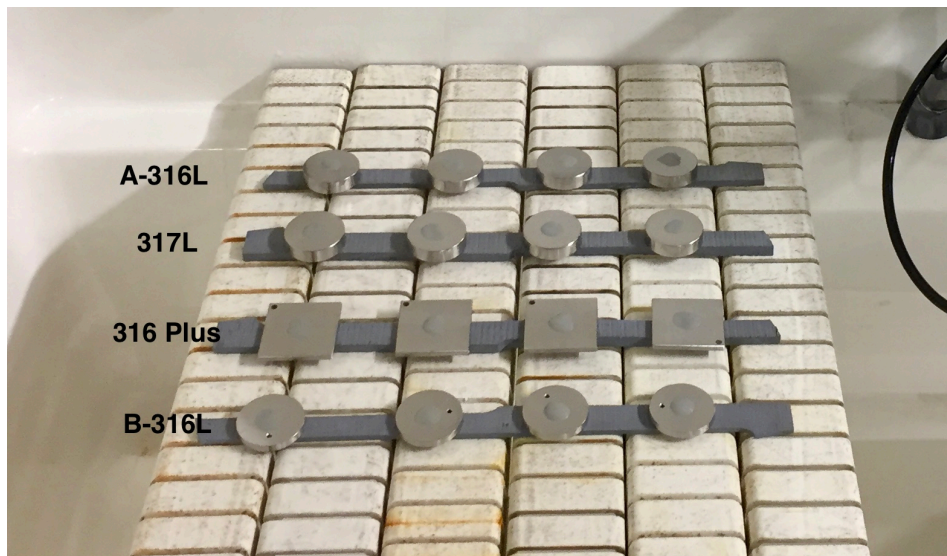
Fig. 4.7: The samples placed in the salt spray chamber.
