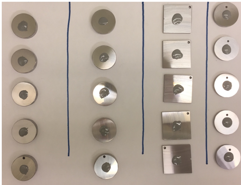
Fig. 4.6: The samples prepared prior to the salt spray exposure and anodic CPP.
