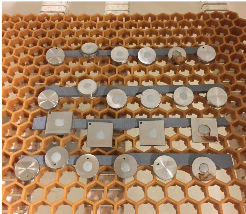
Fig. 5.21: The samples after 67 days in the salt spray chamber at 35 \pm 2 °C with a 5 wt% NaCl salt spray solution. Crevice corrosion was observed on A-316L, B-316L and 316 Plus.
