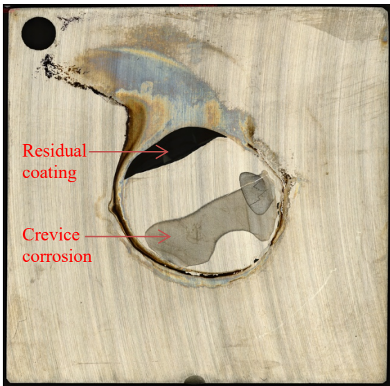
Fig. 5.25: Crevice corrosion attack on 316 Plus after exposure in the salt spray chamber at 35 \pm 2^\circ\text{C} with a 5 wt% NaCl salt spray solution.
