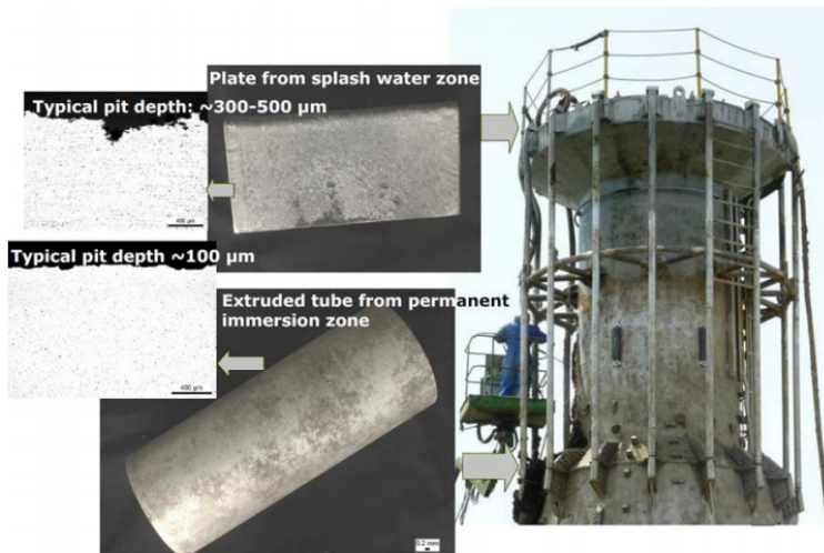
Figure 2.7: North Sea Buoy II after 32 years in seawater.
