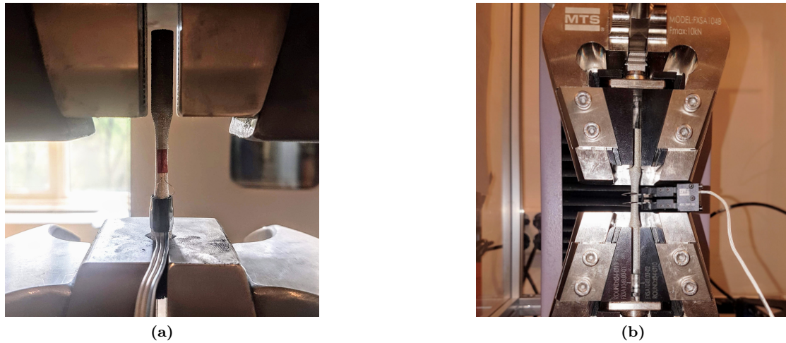
Figure 42: (a) Tensile tests until failure using strain gauges. (b) Tensile test using extensometer at low strain.
