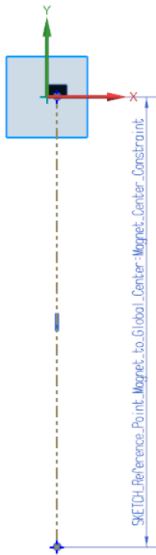
(a) Parametrized reference point for pattern feature and assembly constraints
