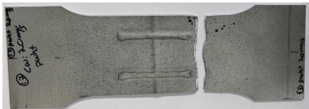
Figure G.6: Fractured specimen with cross weld speed 20 mm/s, with PWHT.
