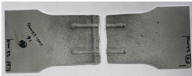
Figure G.7: Fractured specimen with cross weld speed 22 mm/s, without PWHT.
