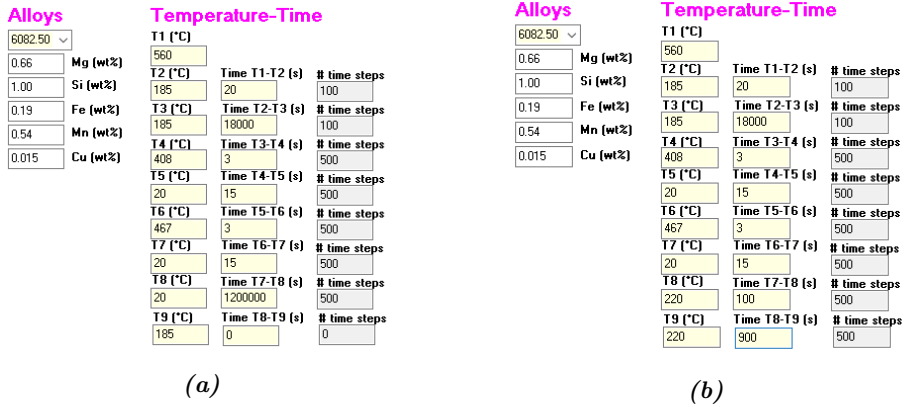
Figure D.3: NaMo input for hardness predictions of welded sheet with 2200 W laser 9 mm from weld center 0.8 mm from the upper surface (through thickness depth = 0.8), where (a) is without PWHT and (b) is with PWHT of 220°C/15min.
