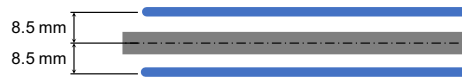
Figure 3.4: Illustration showing the position of the longitudinal laser treatment, indicated by blue lines. The laser treatment was applied to both surfaces of the sheet.
