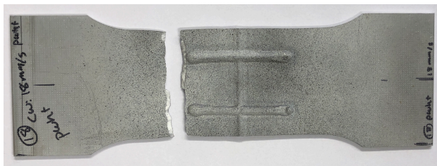
Figure G.4: Fractured specimen with cross weld speed 18 mm/s, with PWHT.
