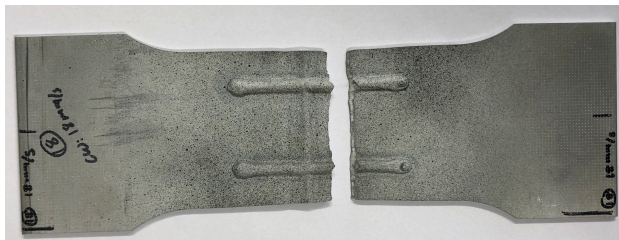
Figure G.3: Fractured specimen with cross weld speed 18 mm/s, without PWHT.
