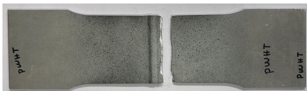
Figure G.12: Fractured specimen with laser pattern, with PWHT.
