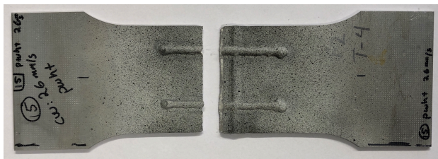
Figure G.10: Fractured specimen with cross weld speed 26 mm/s, with PWHT.
