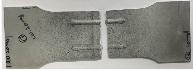
Figure G.5: Fractured specimen with cross weld speed 20 mm/s, without PWHT.
