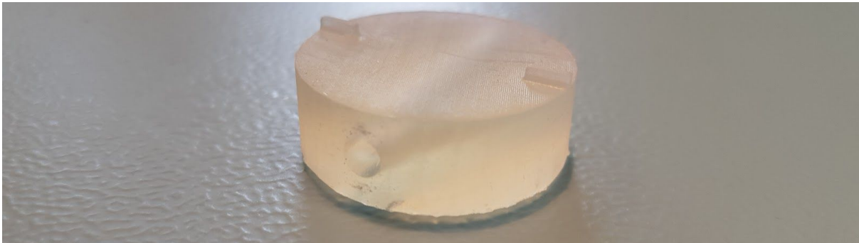
Figure 2: Custom SLA printed notch key
