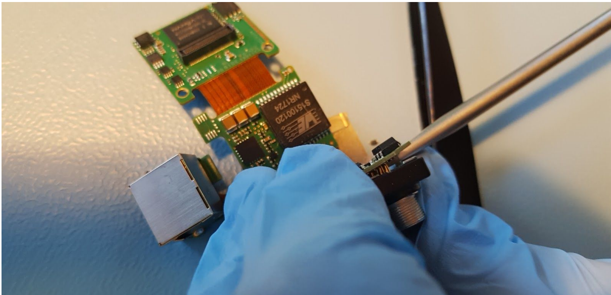
Figure 10. Destructive removal of the I/O eight pin connector
