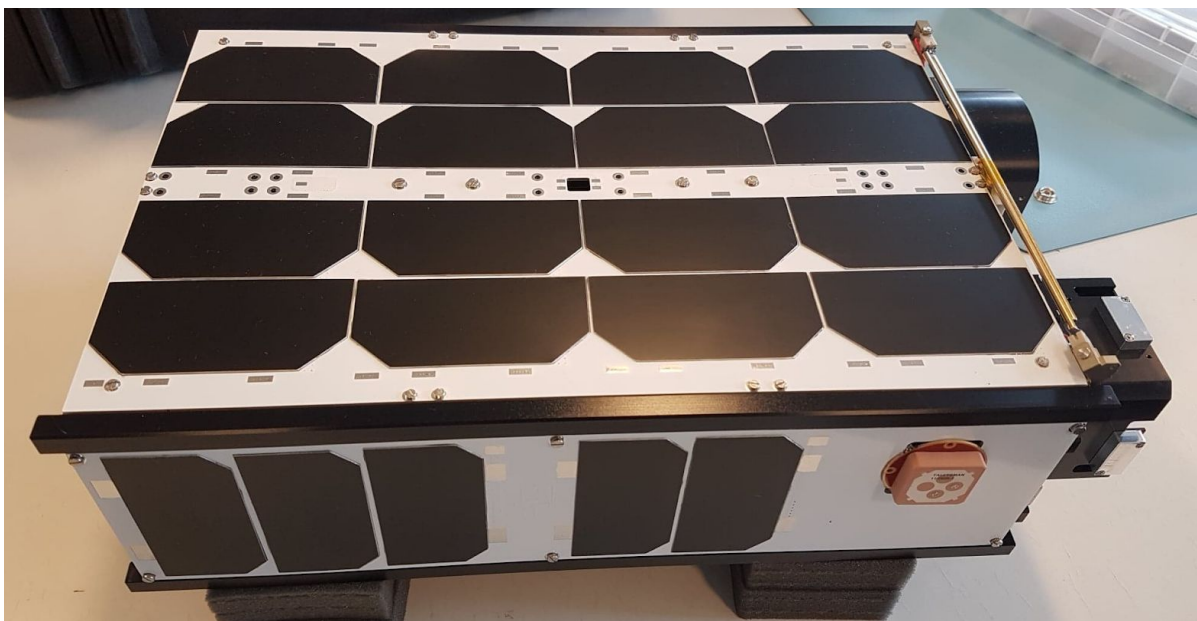
Figure 5: External thermal interfaces, Engineering model from NanoAvionics
