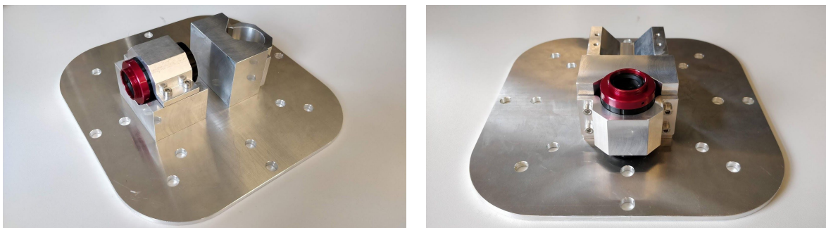
Figure 2: 50mm Objective mounted on the platform in the horizontal position (left), and the vertical position (right)
