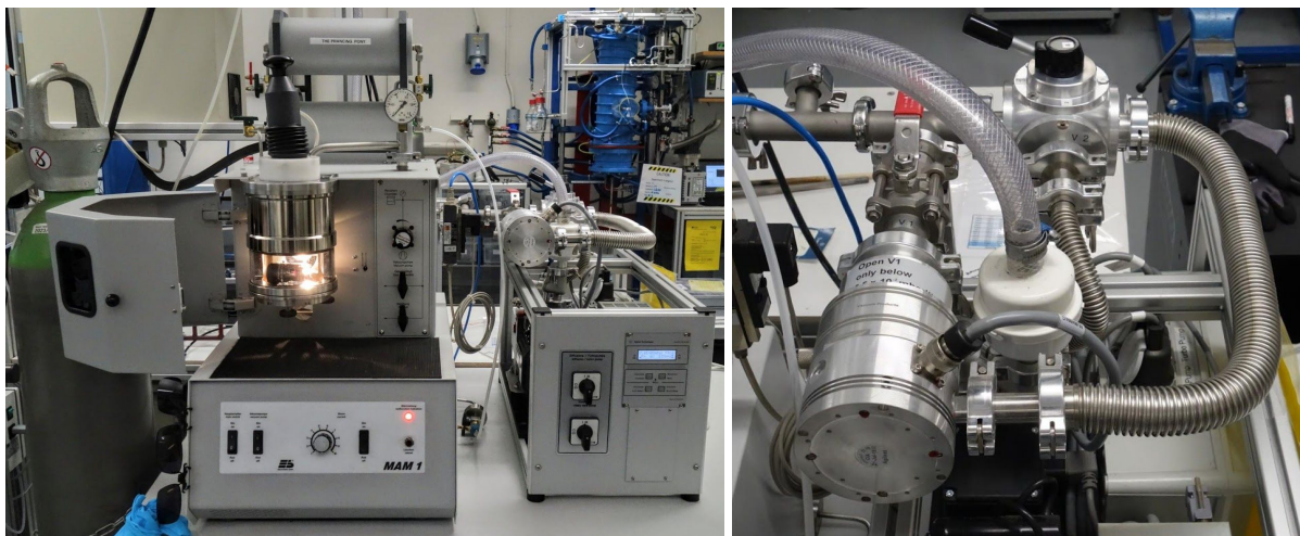
Figure 4: Compact Arc Melter MAM-1 Vacuum Chamber
