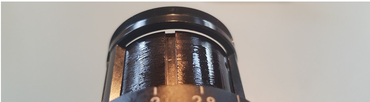
Figure 5: Grease inside the objective
