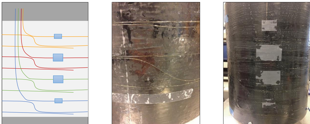
Figure 4 – A: Configuration of optical fibers and Teflon films. B: Turns were kept smooth. C: Four pieces of Teflon film. Two different sizes were used.
