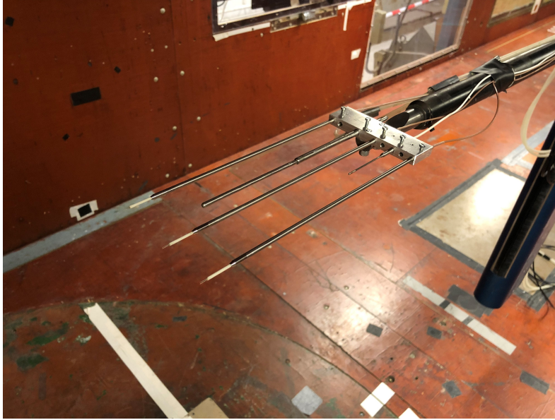
Figure 3.2: Hot wire probes mounted on the traverse.
