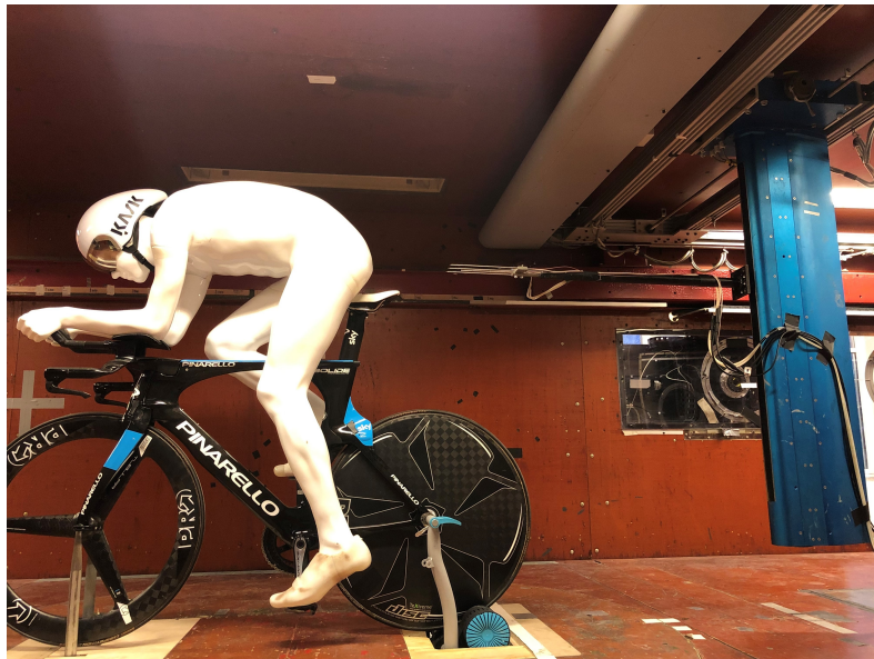
Figure 3.1: Wind tunnel experiment setup includes a full scale mannequin and hot wire probes mounted on the traverse.
