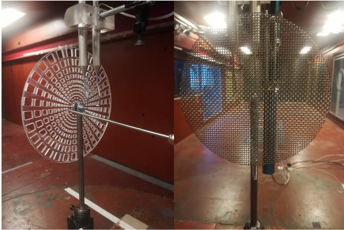
Figure 1. Spider web disk to the left and wire mesh disk to the right. Both disks have a diameter of 20cm and where attached to a mast of D_{mast}/D_{disk} = 0.05
