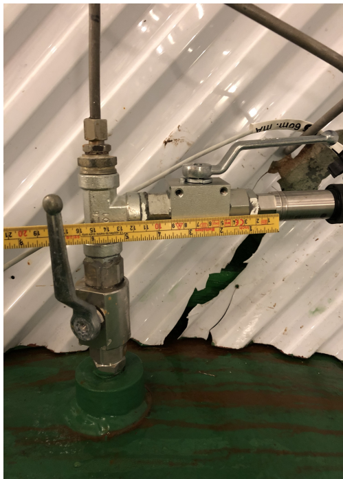
Figure 10.7: Picture of pressure transducer placed upstream the bulb valve, (PU1, PU2, PU3, PU4). The mounting is similar on all the turbines.
