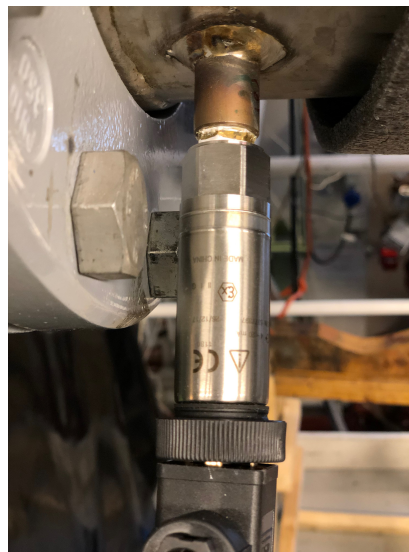
(b) UNIK 5000. Sensor IN3 in Figure 5.3
