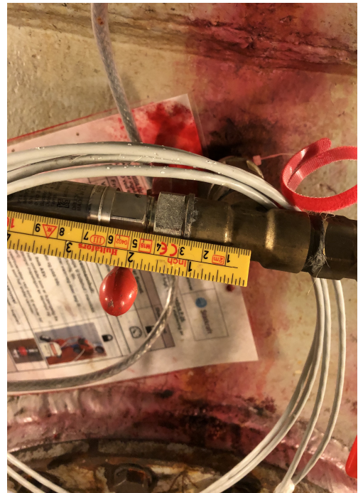
Figure 10.6: Picture of pressure transducer placed on the draft tube of turbine 4.
