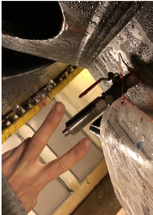
Figure 10.4: Picture of pressure transducer placed on the draft tube of turbine 2.
