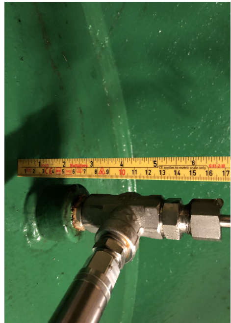
Figure 10.8: Picture of pressure transducer placed downstream the bulb valve, (PD1, PD2, PD3, PD4). The mounting is identical on all the turbines.
