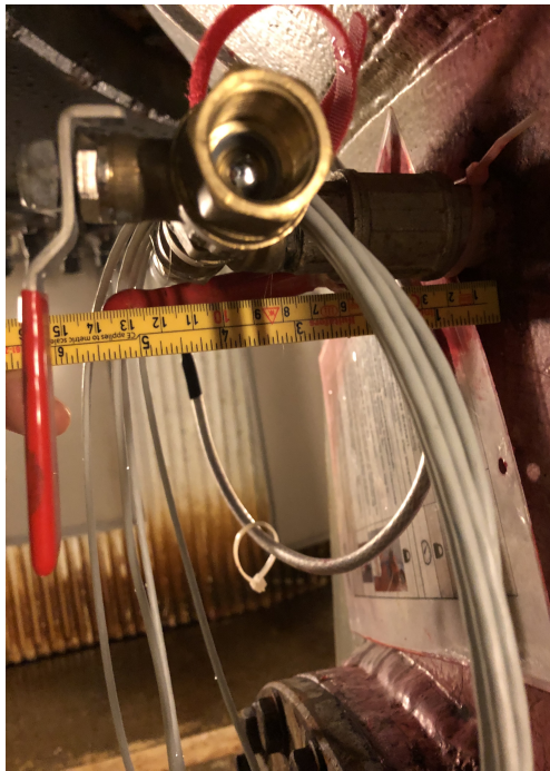
Figure 10.6: Picture of pressure transducer placed on the draft tube of turbine 4.
