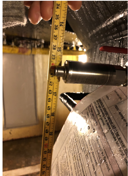
Figure 10.4: Picture of pressure transducer placed on the draft tube of turbine 2.
