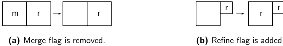
Figure 10: Examples of illegal flag and level combinations, and following countermeasures to avoid size ratio 4. m and r denote the merge and refine flags. The figures are taken from my project report [1], with small changes.
