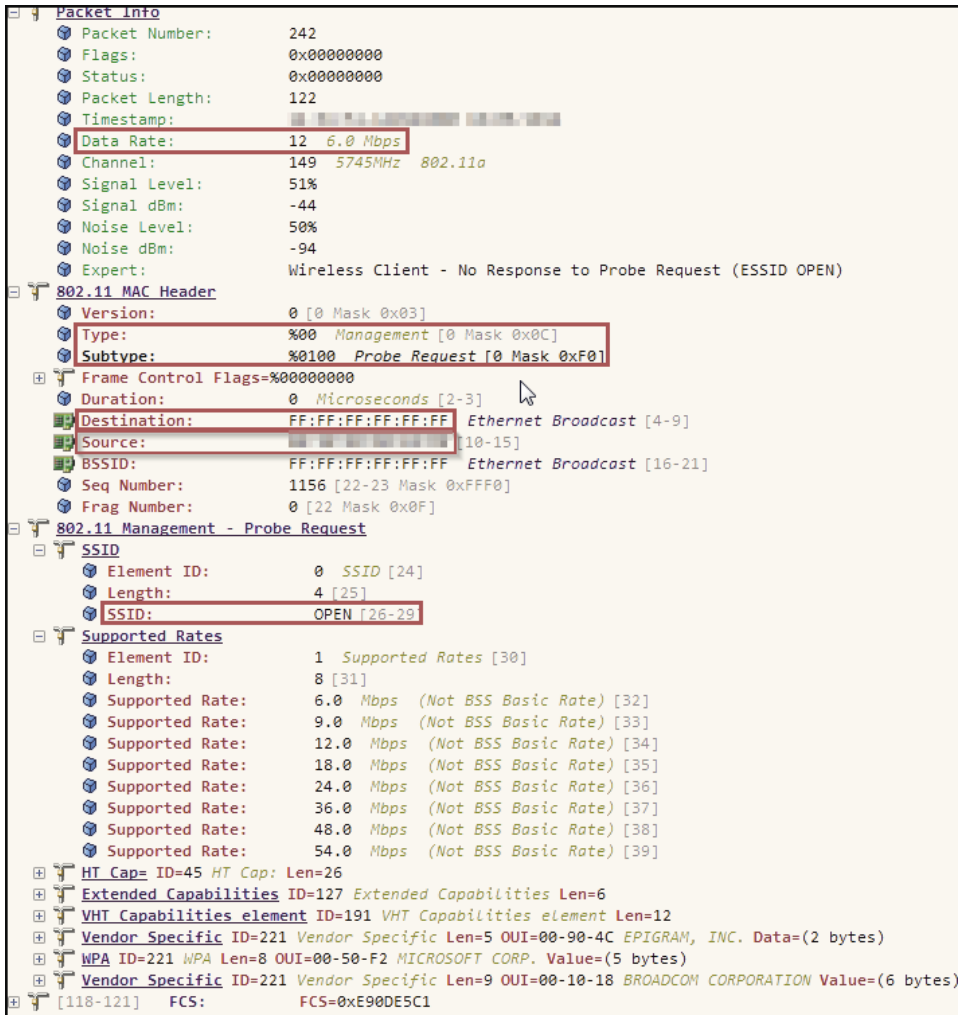
Figure 5.1: Probe request including its real MAC-address.
