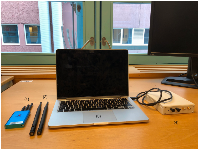
Figure 6.3: Overview of the experimental setup for the illegitimate BTS. 1. Jammer, 2. Vert900 antennas, 3. Macbook Pro running VirtualBox. VM inside VirtualBox running OpenBTS, 4. USRP B210
