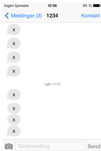
Figure 7.20: Screenshot from Iphone 4s with sysmocom SIM card, showing SMSs received from the LLT 1234 is the number that the LLT SIM card was assigned in OpenBTS
