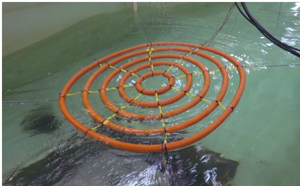
(c) Model moving towards new wave crest, overtopping on 4 tori aft
