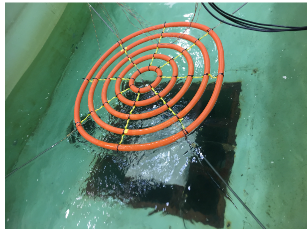
(b) Overtopping follows surface of tori, but disturbs water surface
