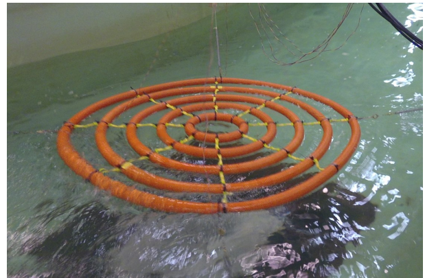
(d) Model moving towards new wave trough, overtopping on 3 outer tori
