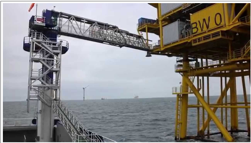
Figure 5.4: Illustration of a W2W gangway [43]
