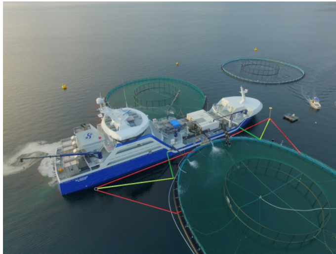
Figure 5.1: Mooring configuration of a wellboat directly moored to the floating collar, (appendix B.2)
