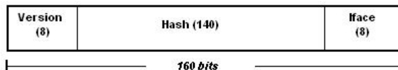
Figure 2.3: AIP address structure.
