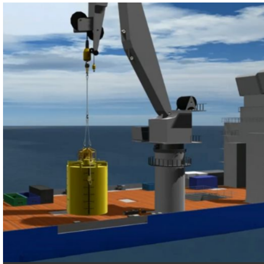
Figure 3.6.4: Suction Anchor on deck of a vessel with installed suction pump (SPT Offshore, 2019)
