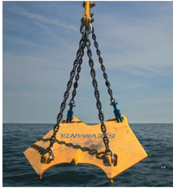
(b) Vertical Loaded Anchor (Vryhof, 2017)
