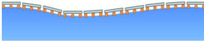
Figur 2.5: Side-view illustrations of the desired global hydrodynamic flexibility of the structure.
