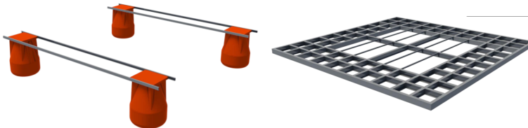
Figur 2.3: Concept illustration of the module frame and floaters
