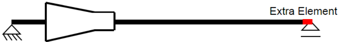
Figure 6.2.5: Illustration of the extra element added for easy application of tension
