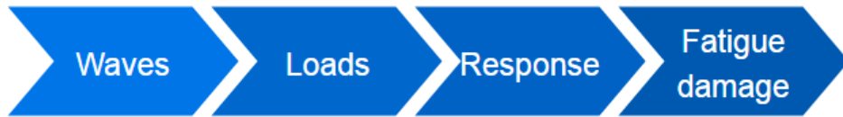
Figure 3.0.1: Flowchart of how waves can give fatigue damage in floating structures
